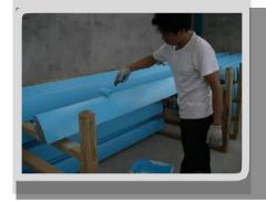
These anodized aluminum bull nose cills were used on the Shanghai Financial Centre. Protectapeel was rolled onto the surface using a lambs wool roller.
